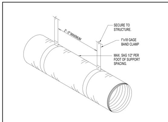
**A FLEXIBLE DUCT SUPPORT** NO SCALE
